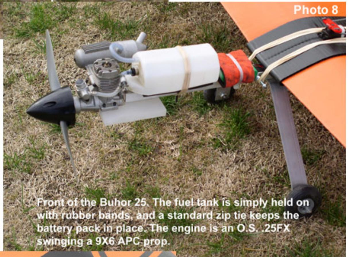
Front of the Buhor 25. The fuel tank is simply held on with rubber bands, and a standard zip tie keeps the battery pack in place. The engine is an O.S. .25FX swinging a 9X6 APC prop.
