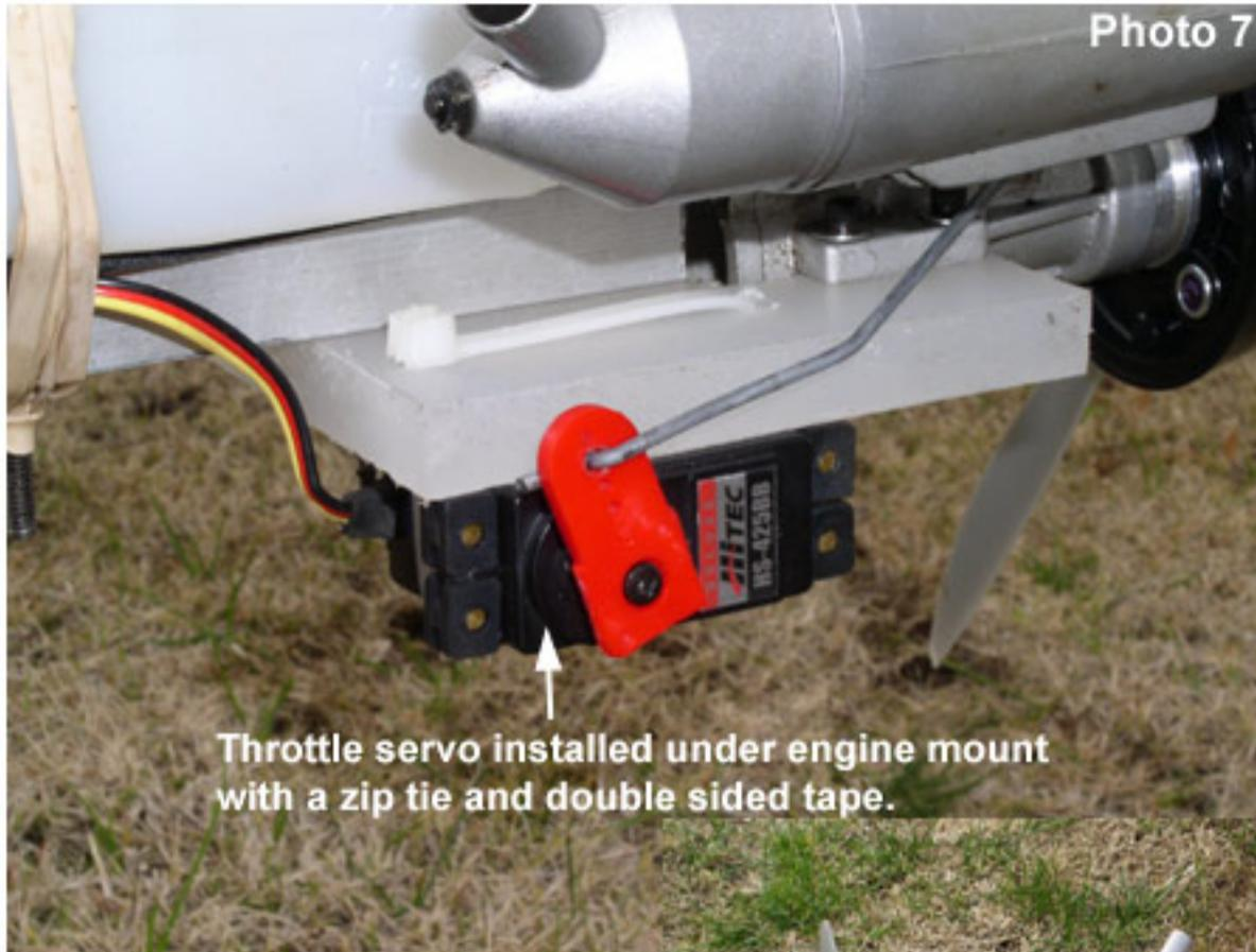
Throttle servo installed under engine mount with a zip tie and double sided tape.
